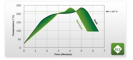
A short 20-30 second soak below the melting point of the solder can be used to help minimize tombstoning.
